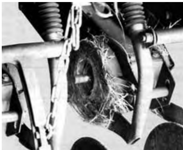
FIGURE 3. Grass Wrapping on Cutter Wheels when Operating in 200 mm (8 in) Prairie Wool.
