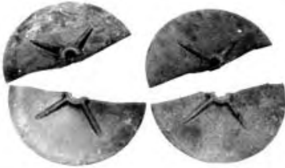
FIGURE 16. Firming Wheel Failure.
