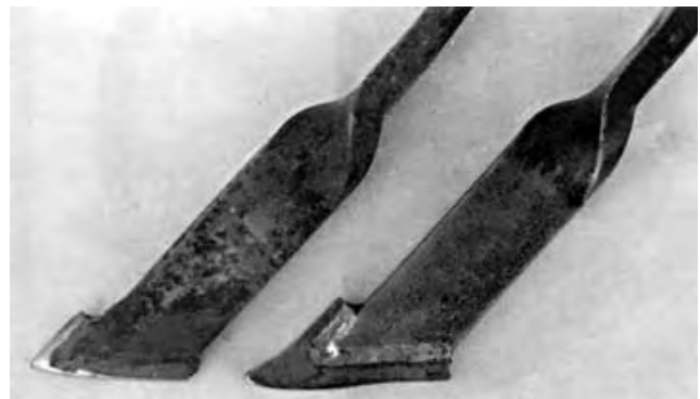
FIGURE 16. Average Wear of the Knife Opener.
