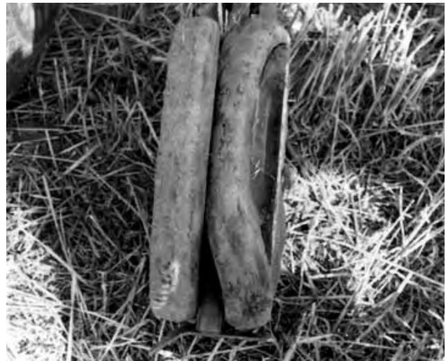
FIGURE 14. Rubber Tire Off Packer.
