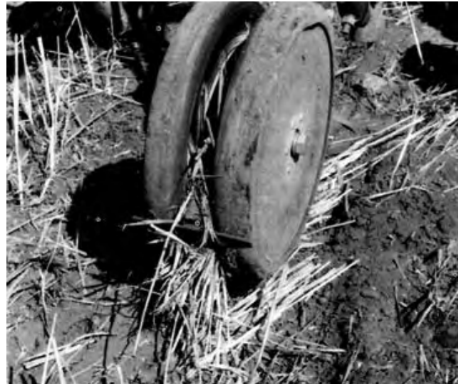
FIGURE 7. Trash Trapped Between Packers at Narrow Spacing.
