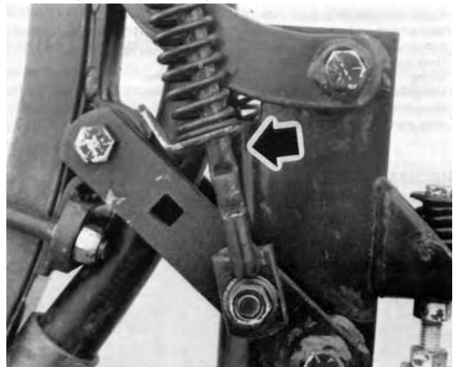
FIGURE 9. Spring Tension Adjustment for Packing Force.
