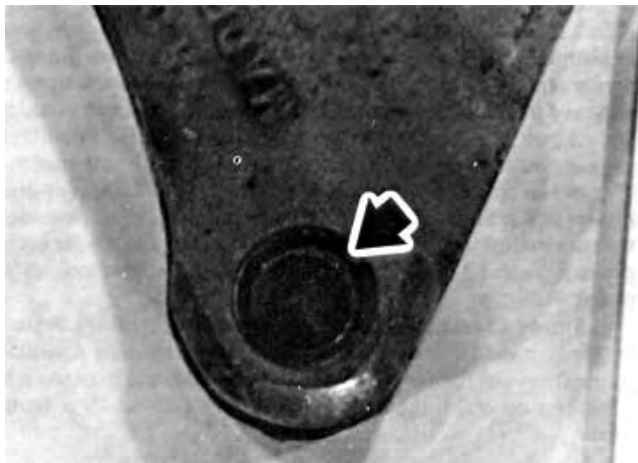
FIGURE 9. Example of Faulty Casting of Double T Slot Adaptor.
