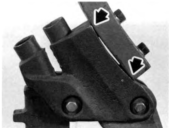
FIGURE 8. Double T Slot Adaptor Made Contact with Shank Only on Top and Bottom.
