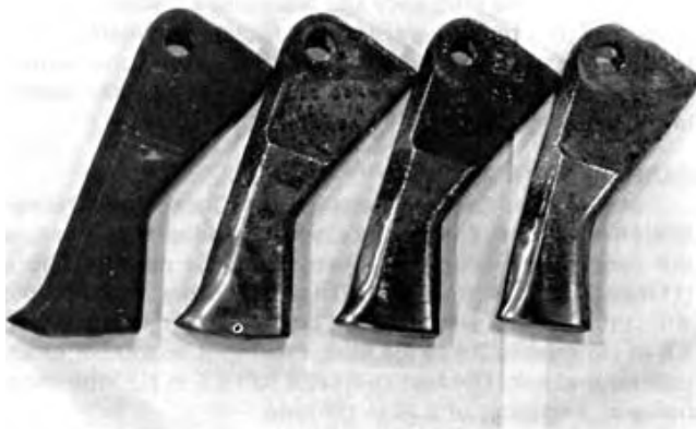
FIGURE 7. Wear on the Banding Blades After 13 ac (5.2 ha) per Blade, 20 ac (8 ha) per Blade and at the End of the Test.
