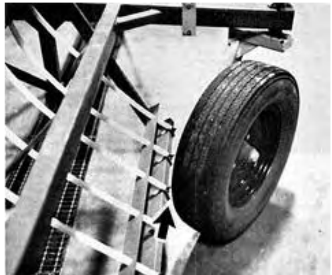
FIGURE 12. Interference Between Front Castor Wheel and Spreader Bar when Turning to the Right in Transport.
