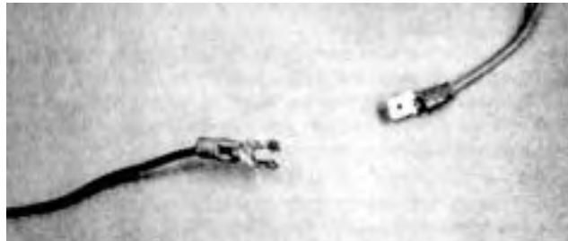
FIGURE 8. Terminals Provided for Connecting Control Panel to the Tractor Battery.
