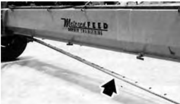
FIGURE 9. Feed Screw Housing Removal for Hopper Cleaning.
