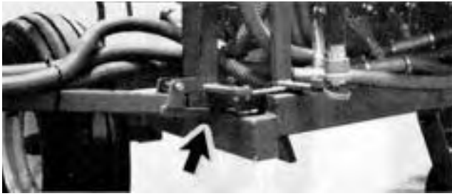
FIGURE 12. Interference Between Stop Bracket and Trailer Frame.
