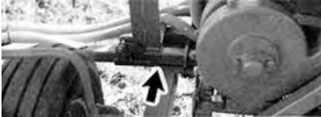
FIGURE 13. Boom Frame Failure.
