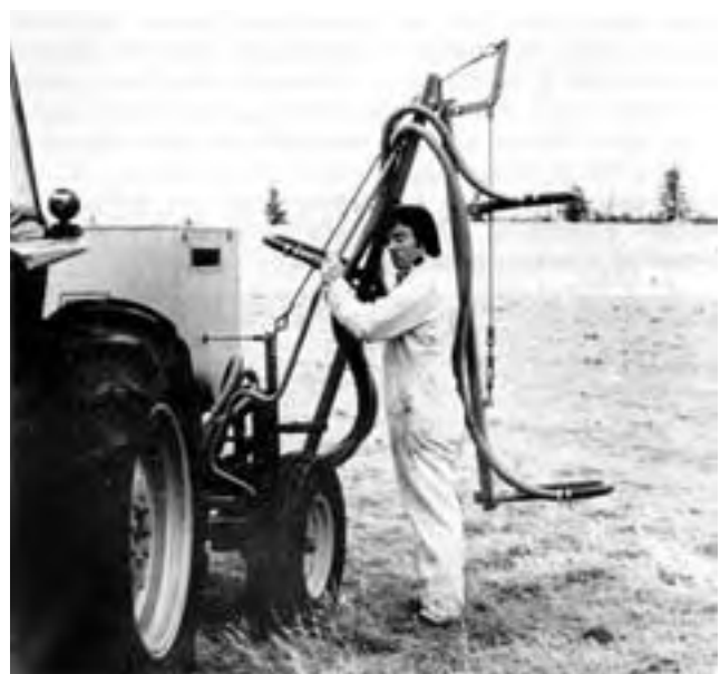
FIGURE 9. Possibility of Being Caught Between Boom Sections when Folding into Transport Position.
