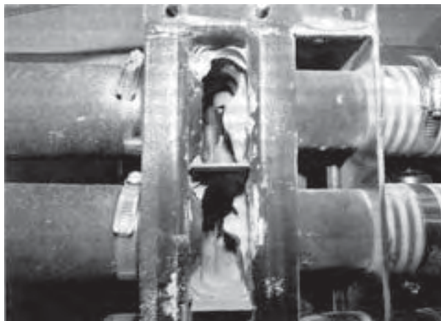
FIGURE 11. Accumulation of Treflan QR5 on the inside of the manifold.
