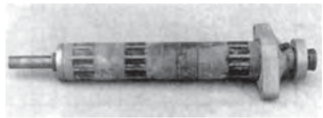
FIGURE 12. Granular Meter Roller.
