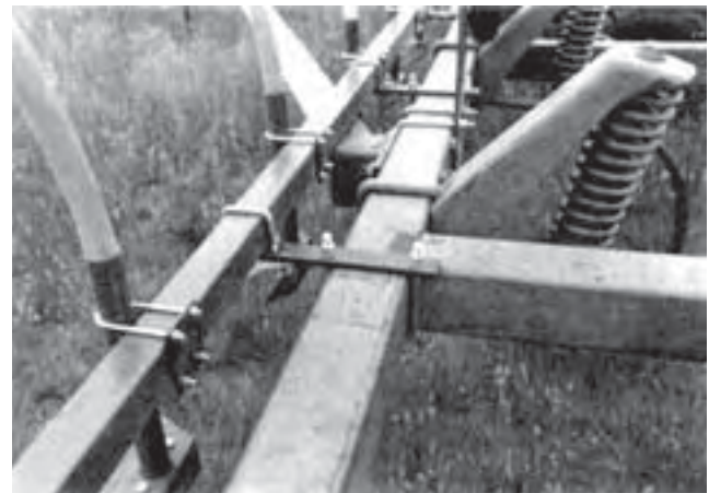
FIGURE 13. Tubing and Spreader Bar Brackets Mounted on Cultivator.
