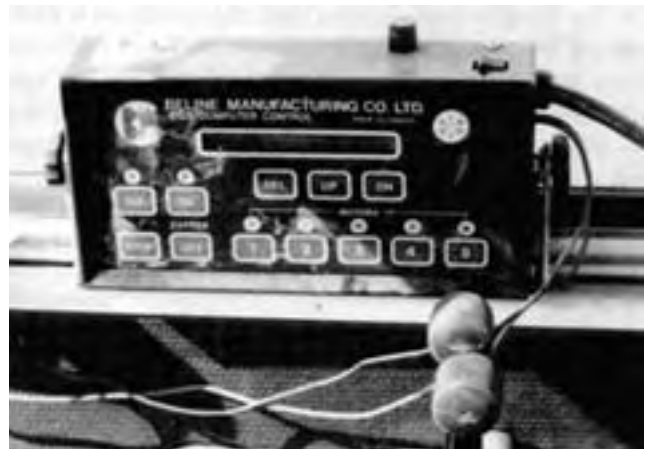
FIGURE 12. Computer Control Located in Tractor Cab.
