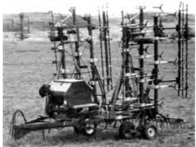
FIGURE 7. Valmar CM240 Mounted on an International Harvester Heavy Duty Cultivator (Upper: Field Position, Lower: Transport Position).
