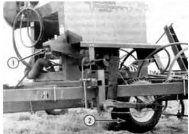
FIGURE 8. (1) Meter Gear Box, (2) Ground Drive Wheel.
