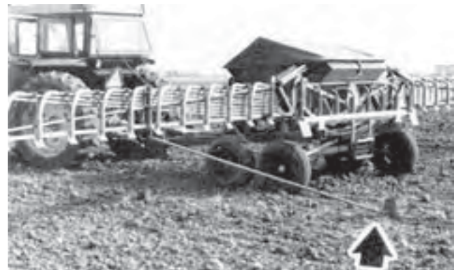
FIGURE 7. Disc Marker Flipped Backwards out of Position.
