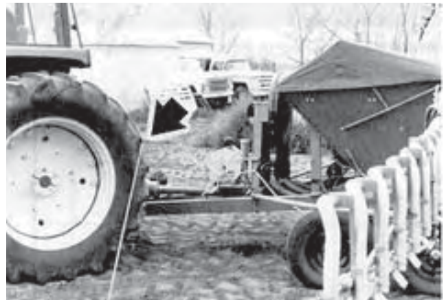
FIGURE 8. Disc Marker Cable and Tractor Tire Interference.
