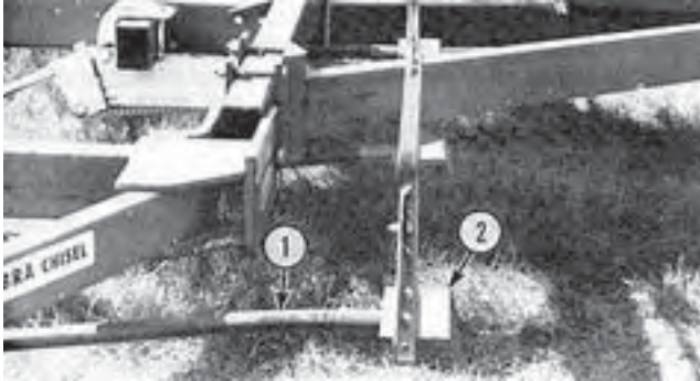
FIGURE 4. Distribution System: (1) Outlet Hose, (2) Deflector Plate.
