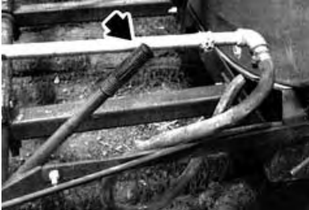
FIGURE 20. Interference Between Boom Adjusting Handle and Right Boom in Transport.
