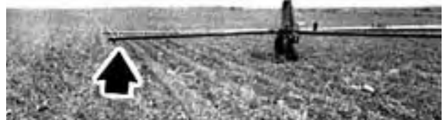
FIGURE 19. Sagging Boom End.
