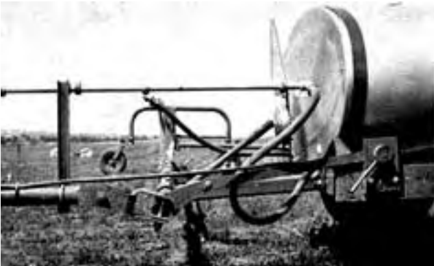
FIGURE 21. Adjusting Handle Set Ahead to Avoid Interference but Universal Joint Angled Up.
