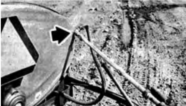
FIGURE 22. Interference Between Boom and Tank.
