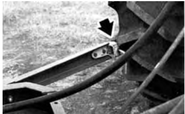
FIGURE 17. Interference Between Radius Rod Bracket and Tractor Tire.
