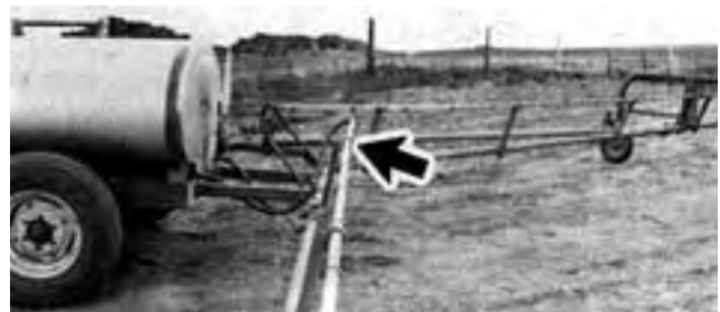
FIGURE 18. Slight Bending at Inner End of 64 mm (25 in) Boom Support Rail Assembly.
