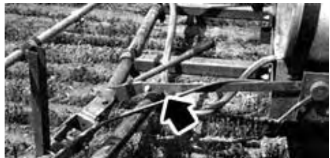
FIGURE 16. Interference Between Radius Brace and Boom Adjusting Linkage.
