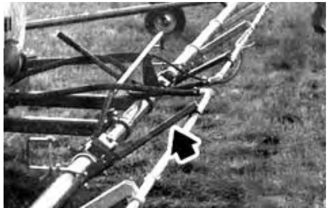
FIGURE 12. Extra Support at Inner Ends of 76 mm (3 in) Boom Support Rail Assembly.
