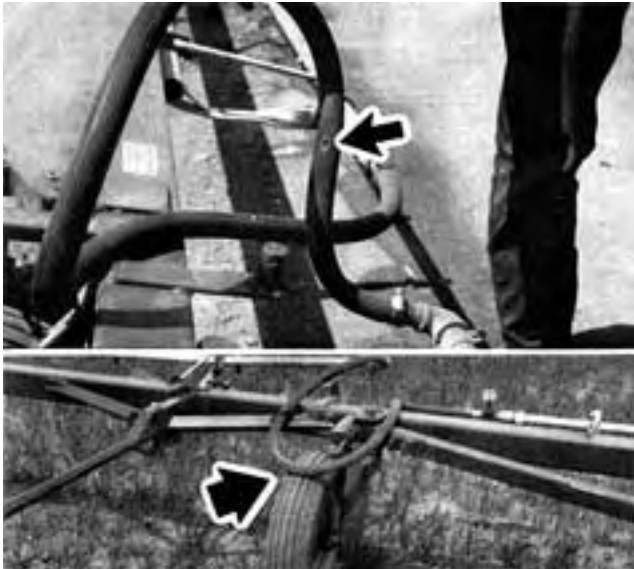
FIGURE 16. Boom Extension Hose Wear Due to Rubbing on Frame and Tires.
