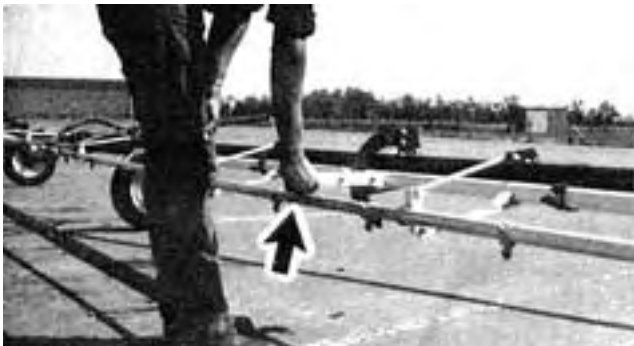
FIGURE 14. Fingers Pinched Between Boom Adjusting Handle and Boom when Placing the Boom in Field Position.
