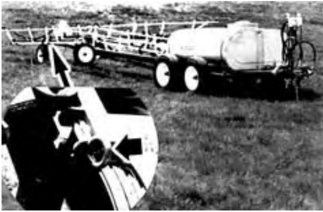
FIGURE 13. Wilger 804S Folded into Transport Position Showing Detail of Boom Wheel Lock Pin.
