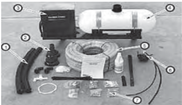
Figure 17. Richway Industries Model SG3013 Foam Marker 1) Foam Discharge Tubes, 2) Foam Discharge Boots, 3) Compressor, Filter and Control Valve Housing, 4) Foam Tank, 5) Foam Carrier Hoses, 6) Foam Tank Cap and 7) Hardware.
