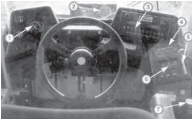
Figure 13. Spra Coupe's Console Layout (1) Instrumentation Console (2) Pressure Gauge (3)Raven Spra controller Console (4)Foam Marker Controls (5) Hand Throttle Lever (6) Boom Control Console and (7) Shift Lever.
