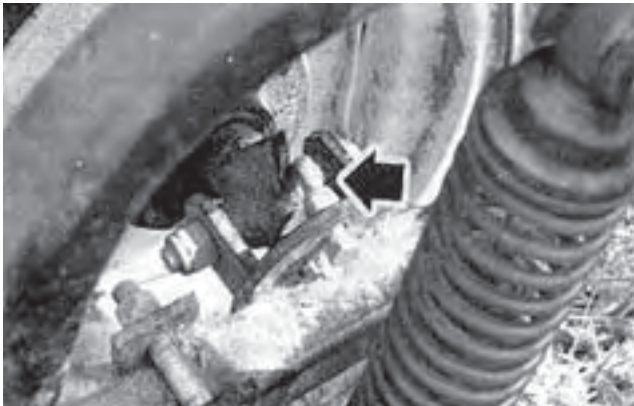
FIGURE 15. Bent Castor Wheel Camber Adjustment Bolts.
