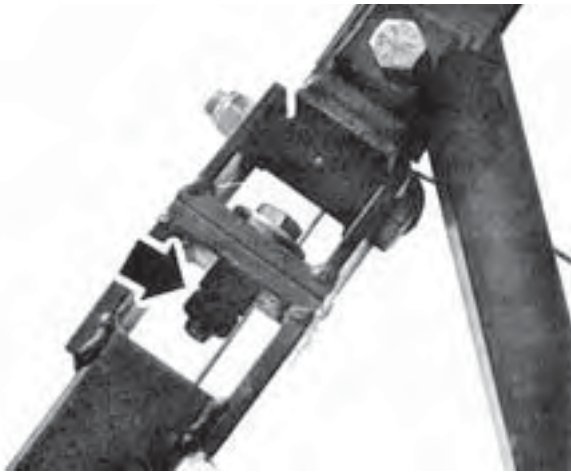
FIGURE 14. Loose Outer Boom Radius Arm Bolts.
