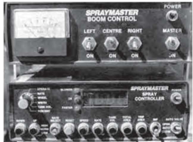
FIGURE 14. Computronics International Remote Control (upper) and Automatic Application Rate Controller Consoles (lower).
