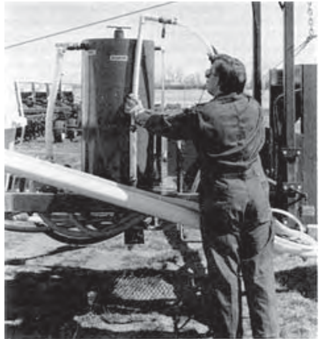
FIGURE 17. Operator Using Chemical Inductor Wand.
