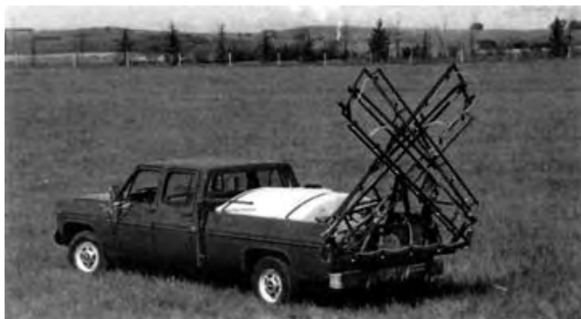
FIGURE 10. Sprayer in Transport Position.
