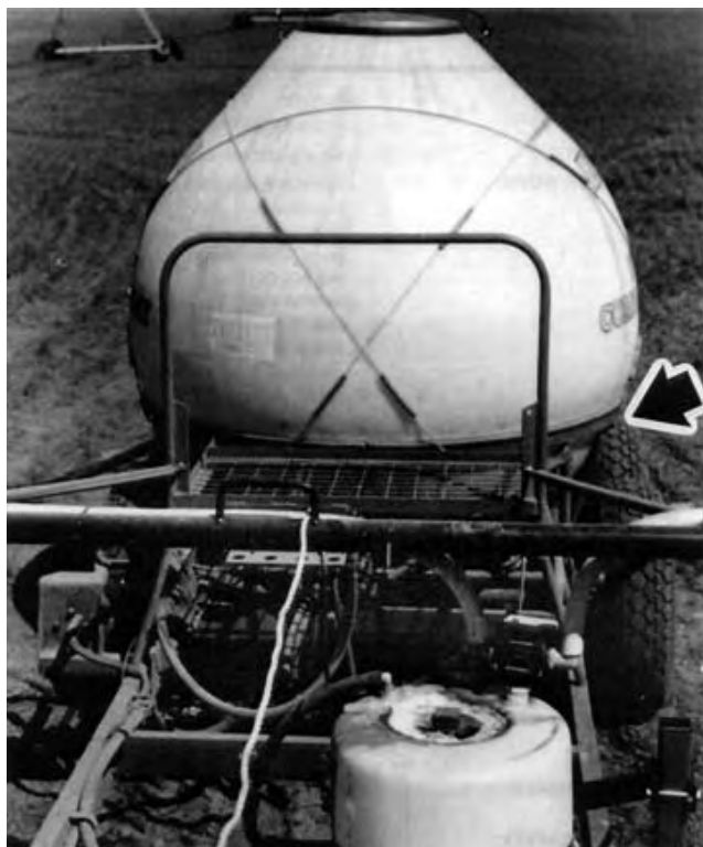
FIGURE 9. Operator's View of S.S.C.I.M.S. Completely Obscured by Sprayer Water Tank. Arrow Indicates Location of Injector Pump.
