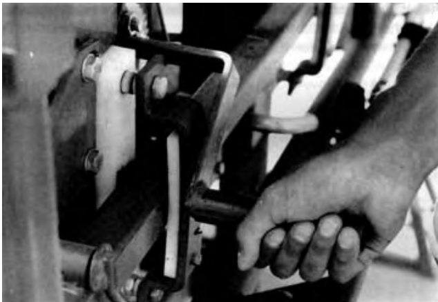
FIGURE 12. Winch Crank and Boom Frame Interference.
