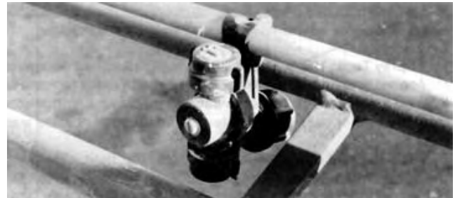
FIGURE 9. Application Rate Control System: (1) Pressure Gauge Green Zone, (2) Application Rate Decal, (3) Control Valve.
