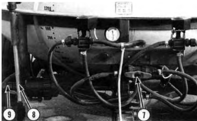
FIGURE 1. Vicon Model LS 2340T Field Sprayer: (1) Liquid Level Indicator, (2) Spray Tank, (3) Self-Stabilizing Boom System, (4) Spray Boom, (5) Main and Agitator Pumps, (6) Nozzle Body Assembly, (7) Sprayer Control System, (8) Chemical Inductor, (9) Reload System.
