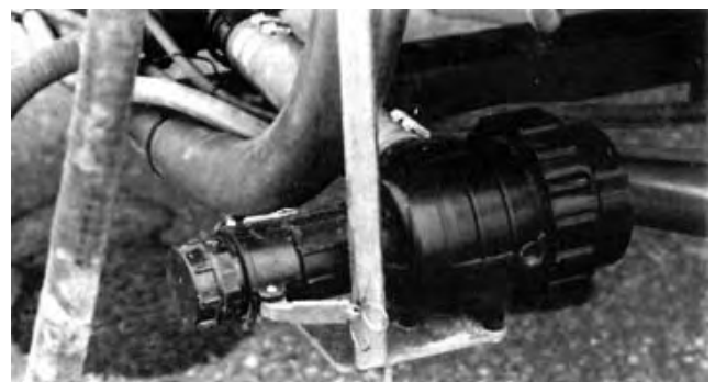
FIGURE 15. Chemical Inductor Tube and Reload Inlet Coupler Interference.
