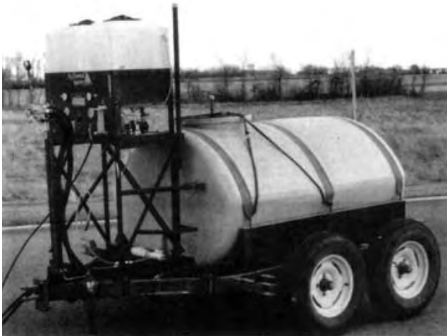
FIGURE 2. Ag-Chemical Injector on Elevated Framework for Improved Visibility from Tractor Cab.
