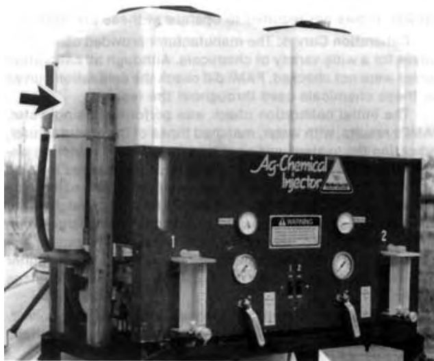
FIGURE 5. Graduated Cylinder Mounted on the Ag-Chemical Injector to Assist in Field Calibration.
