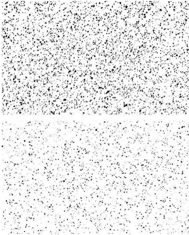
FIGURE 20. Droplet Sizes Produced by the Micromax when Spraying at the Medium Speed (4500 rpm) (Upper: 4916-37 Orifice Plate, Lower: 4916-26 Orifice Plate).
