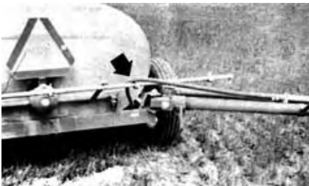
Figure 14. Boom Hose Caught on Nozzle Clamp.
