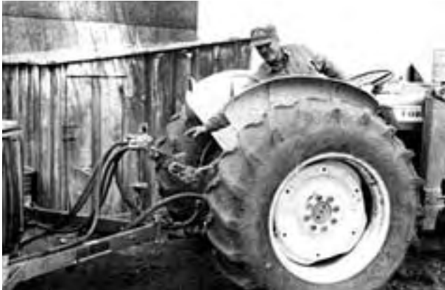
Figure 12. Awkward Location of Controls.
