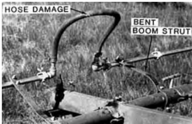
Figure 26. Damaged Boom Extension Hose and Bent Boom Strut.
