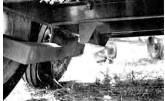
Figure 17. Damage to Rocker Axle.
