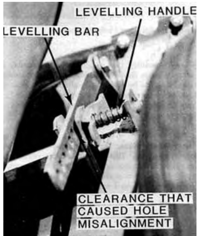
Figure 15. Boom Height Adjustment Mechanism.
