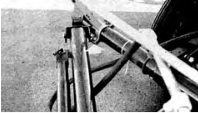
Figure 20. Short Turn in Transport causing Bending of the Boom Universal Joint.
