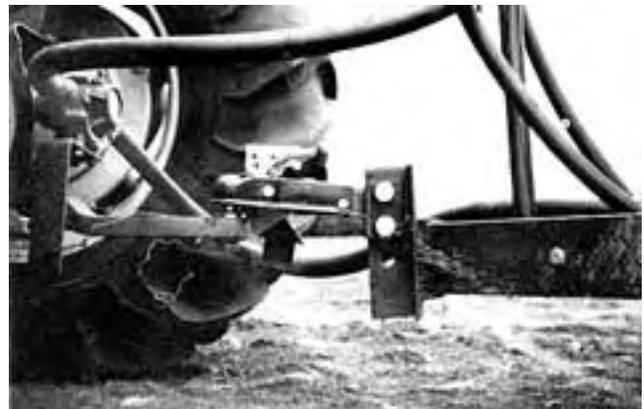
Figure 16. Weak Ball Joint Coupler.
