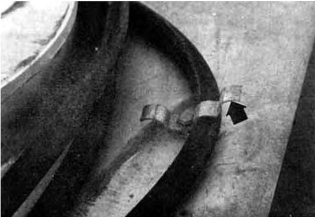
Figure 19. Hose Holder Deformation.
