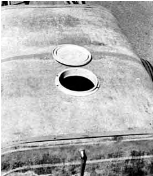
Figure 18. Location of Tank Filler Opening.
