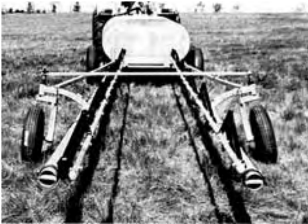
Figure 17. Excessive Camber of Castor Wheels.
