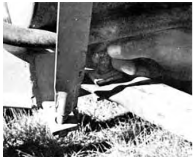
Figure 16. Awkward Location of Radius Brace Pin.
