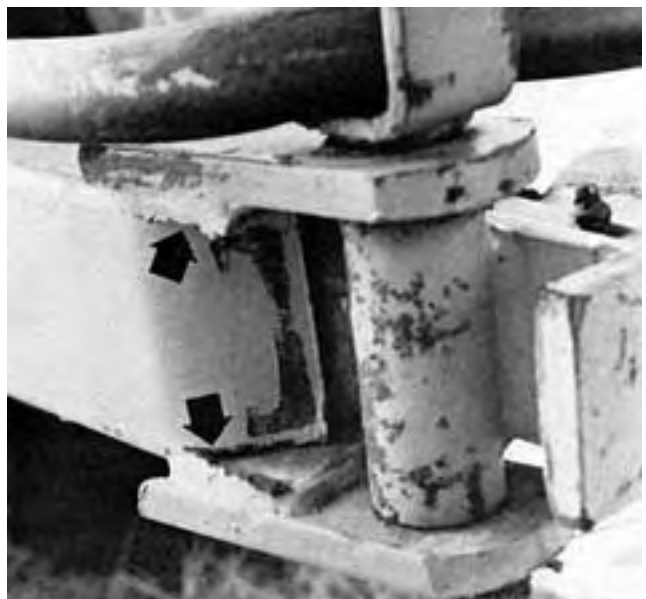
Figure 24. Failure of Trailer Frame.
