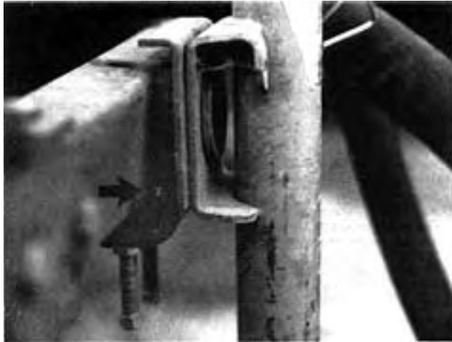
FIGURE 19. Nozzle Angle Pointing Back After Radius Mounts Shifted Downwards.
