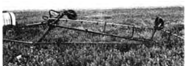
FIGURE 22. Rotation of Tandem Beam Assembly Around the Boom Rail.
