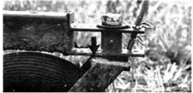
FIGURE 20. Hitch Jack Inadequately Secured.
