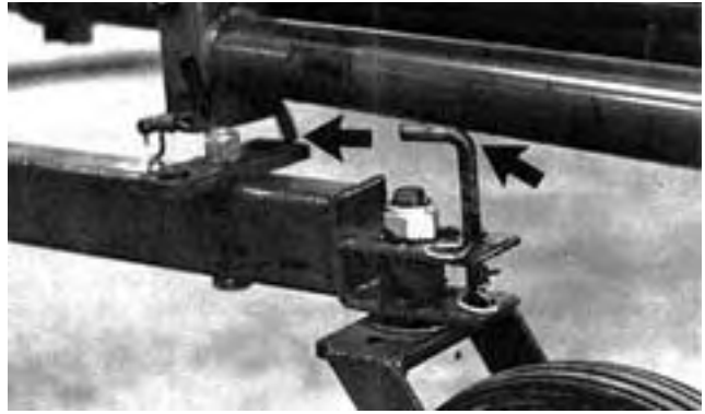
FIGURE 15. Interference Between Boom Rail, and Outer Radius Rod Pins.
