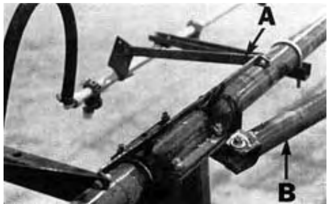
FIGURE 16. Interference Between Outer Radius Rod and Outer Tandem Beam Assembly.
