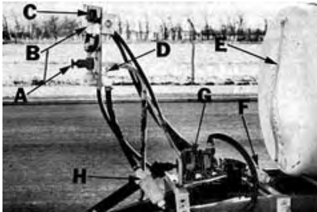
FIGURE 11. Controls: (A) Boom Control Valve, (B) Solenoid Valves, (C) Pressure Gauge, (D) Agitator Valve, (E) Liquid Level Indicator, (F) Shut-off Valve, (G) Pump, (H) Line Strainer.
