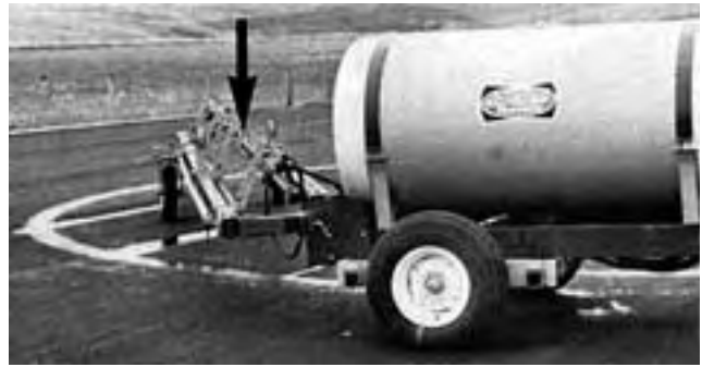
FIGURE 12. Boom Interference when Making Sharp Turns.
