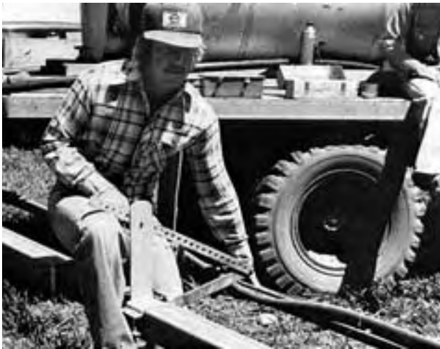
FIGURE 14. Operator Aligning Nozzle Height, Adjusting Bar with his Knee.
