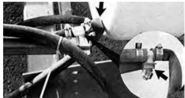
FIGURE 15. Interference Between Tank and Middle Boom Inlet Hose Causing End Nozzle Damage.
