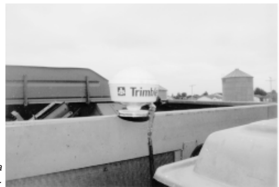
Ag Leader antenna positioned on a John Deere 7720 combine.
