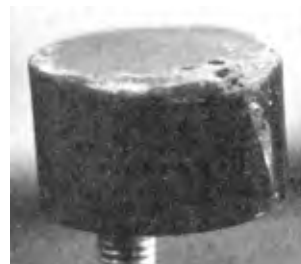
FIGURE 10. Damaged Speed Sensor.
