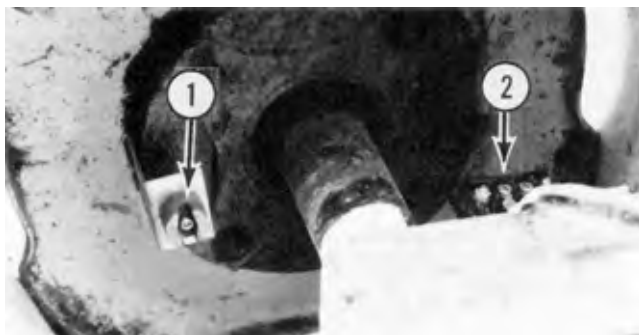
FIGURE 2. Wheel Transducer: (1) Magnet, (2) Detector Switch.
