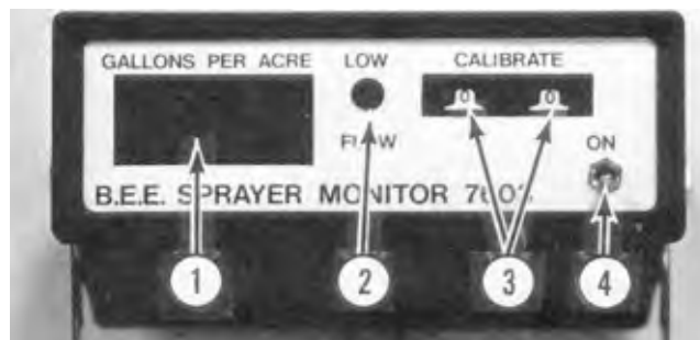
FIGURE 3. BEE Meter: (1) Application Rate Display Screen, (2) Low Flow Indicator Light, (3) Calibration Thumbwheel Switches, (4) On-Off Power Switch.
