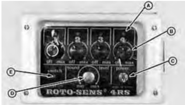
FIGURE 2. Control Box: (A) channel warning lights, (B) speed adjustment dials, (C) power switch, (D) buzzer sound level adjustment, (E) alarm switch light.
