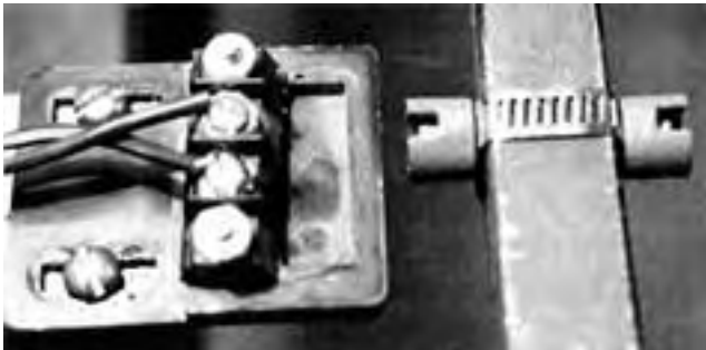
FIGURE 3. Slow Speed Detector, With Magnets Attached to a Drill Seed Shaft.
