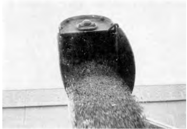
FIGURE 8. Grain Flow Over Top of Grain Flow Sensor Baffle.
