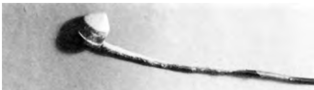
FIGURE 3. Powder Buildup on Sensor Face.
