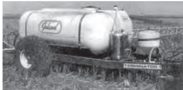
FIGURE 6. Foam Tank and Compressor Housing.
