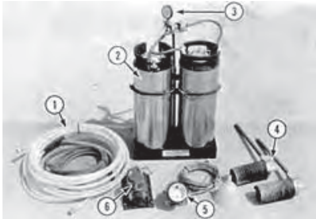
FIGURE 1. Marshall Model 5520 Foam Marker: (1) Foam Tubes, (2) Foam Tank, (3) Pressure Gauge, (4) Boom End Funnels, (5) Control Console, (6) Compressor.
