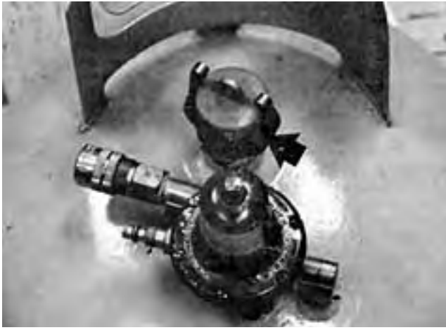
FIGURE 4. Filler Cap on Supply Tank.
