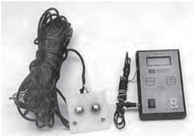
FIGURE 4. Delmhorst RDM-H Forage Moisture Tester.
