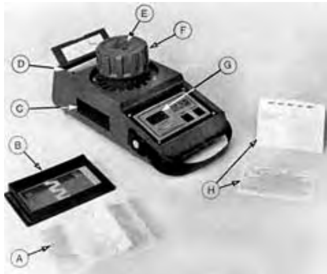
Figure 1. (A) Forage Sample Bags, (B) Grain Sample Tray, (C) Sample Chamber, (D) Storage Compartment, (E) Pressure Indicator, (F) Pressure Control Knob, (G) Digital Display, (H) Moisture Conversion Tables.
