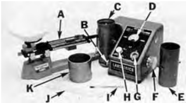
FIGURE 1. Labtronics 919 Grain Moisture Meter: (A) Triple Beam Balance, (B) Adjust Knob, (C) Cell, (D) Meter, (E) Dump Cylinder, (F) Dial Knob, (G) Dial Reading, (H) Function-Calibrate Knob, (I) Thermometer, (J) Rapeseed Counter, (K) Pint Measure.
