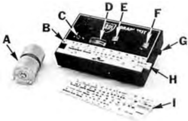
FIGURE 1. RDS Grain Test 2 Moisture Meter: (A) Test Cell, (B) Meter Scale, (C) Power Switch, (D) Meter Indicator, (E) Meter Reading, (F) Temperature Reading, (G) Built-in Temperature Sensor, (H) Sliding Crop Scale, (I) Additional Crop Scales.
