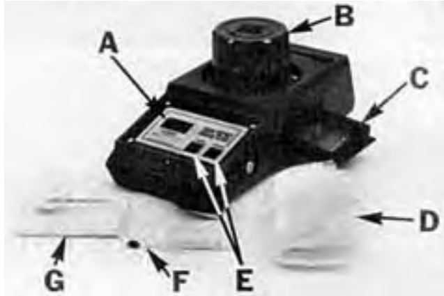
FIGURE 1. Froment NJF 1210 Moisture Tester: (A) Digital Readout, (B) Pressure Control Knob, (C) Grain Sample Tray, (D) Forage Sample Bags, (E) Control Buttons, (F) Thermometer, (G) Moisture Charts.
