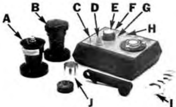
FIGURE 1. Protimeter Grainmini III Moisture Meter: (A) Grinder, (B) Compressor, (C) Switch, (D) Calibration Knob, (E) Meter Dial, (F) Calibrate Light, (G) Meter Scale, (H) Read Light, (I) Reader Rings, (J) Grain Cell.
