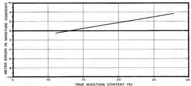
Figure 4. Deviations of Meter Readings for the Labtronics 919 in Oats.
