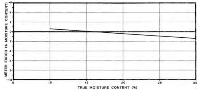
Figure 3. Deviations of Meter Readings for the Labtronics 919 in Barley.
