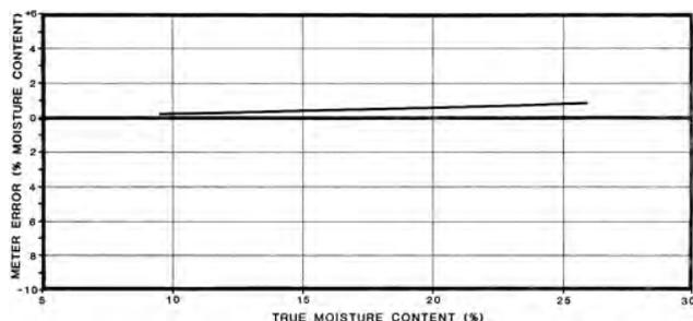
Figure 2. Deviations of Meter Readings for the Labtronics 919 in Wheat.
