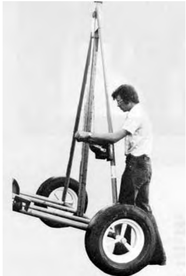
FIGURE 2. Inconvenient Winch Handle Location.
