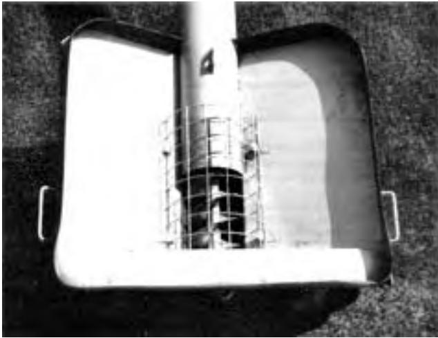
FIGURE 4. Inlet Hopper and Safety Guard.
