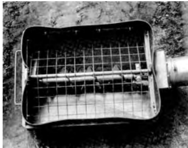
FIGURE 4. Inlet hopper and safety guard.
