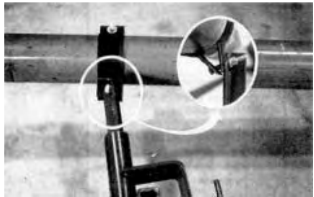
FIGURE 2. Truck mount (auger clamp fastened to the angle support shown in inset) The truck box clamp made installing the Blanchard simple on most truck boxes.
