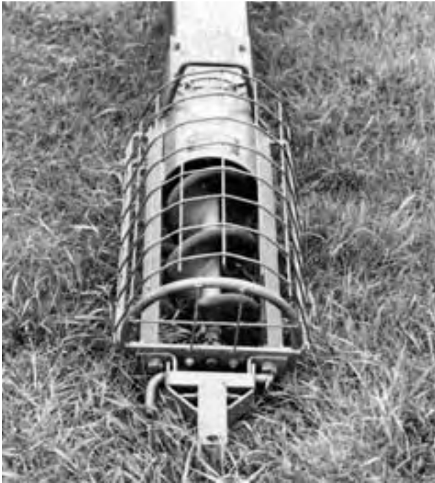
FIGURE 5. Inlet safety guard.
