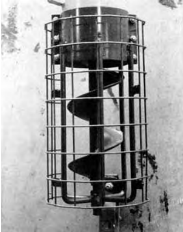
FIGURE 5. Inlet Safety Guard.
